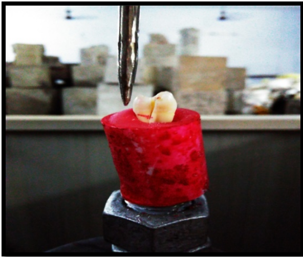
Figure 8: Fracture resistance tested under universal testing machine
