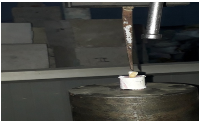
Figure 15: Load applied over the prepared tooth
